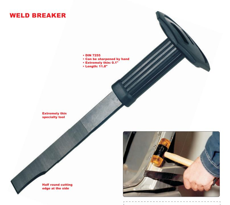
This spot weld breaker is meant to replace or reskin body panels and frame sectioning. It is inserted between seams or panels after spot welds are drilled out to completely remove panel sections. A treated steel shank with an extremely thin, half-rounded cutting edge finishes the separation process. This tool stores inside the handle for safety, with a simple cross guard to protect your hand. The smooth blade ensures that you have full control.
