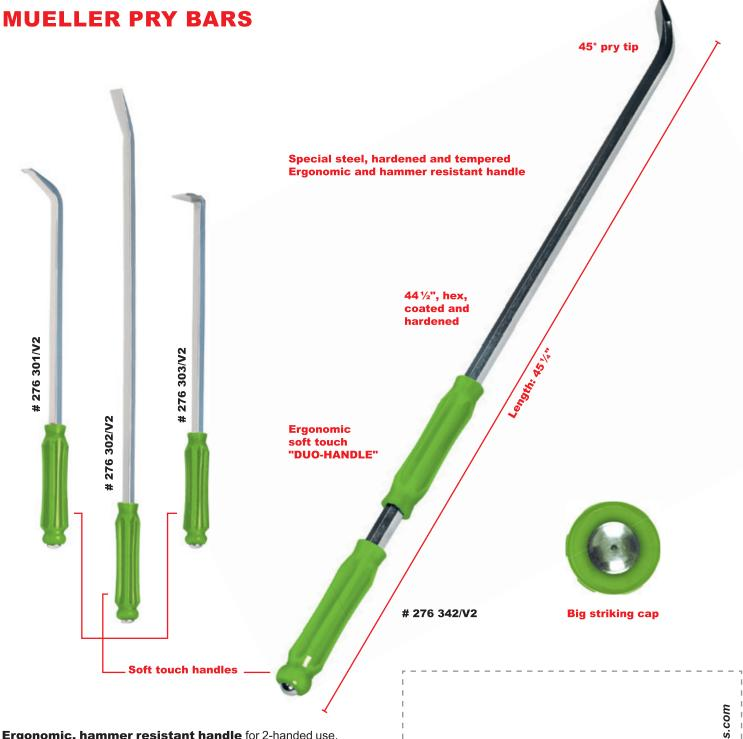
**Ergonomic, hammer resistant handle** for 2-handed use. Special steel 16x16mm going through the handle, large striking cap for tough daily jobs. Soft touch handles. Made for heavy duty jobs such as trucks and offshore work.
