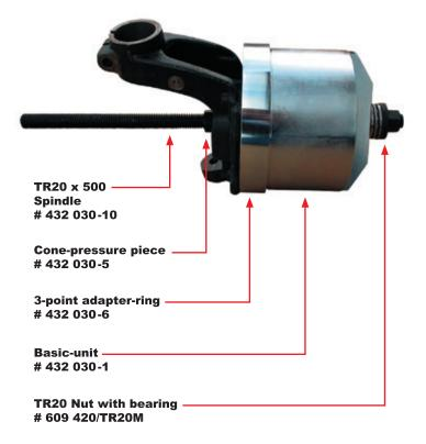
Suitable for almost all vehicles with bearing hub units (compact bearings) as well as with conventional wheel bearings.
