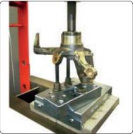
**Universal tool set for pressing in and out** wheel bearings, bushings, shaft seals etc.
