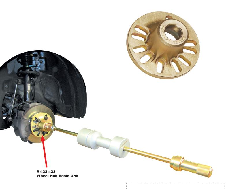
The Wheel Hub Basic Unit is drop forged for exceptional strength. Suitable for 4 and 5 lug applications. To be used with the 433 450 XL Slide Hammer.
