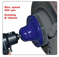
**Special grinder for cleaning the wheel centering device** and the attachment face between WHEEL and HUB. Stubborn corrosion residue is removed quickly, easily and completely. Optimized for use with an Impact gun. Actual processing time per hub 3 - 25 seconds. Works best at lowest rpm.
