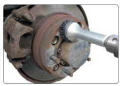
Special grinder used to clean the wheel rim contact surface, designed for vehicles with stud bolts. Corrosion is quickly and easily removed.
