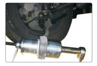
Sleeves outer diameter from: 44 - 82 mm
