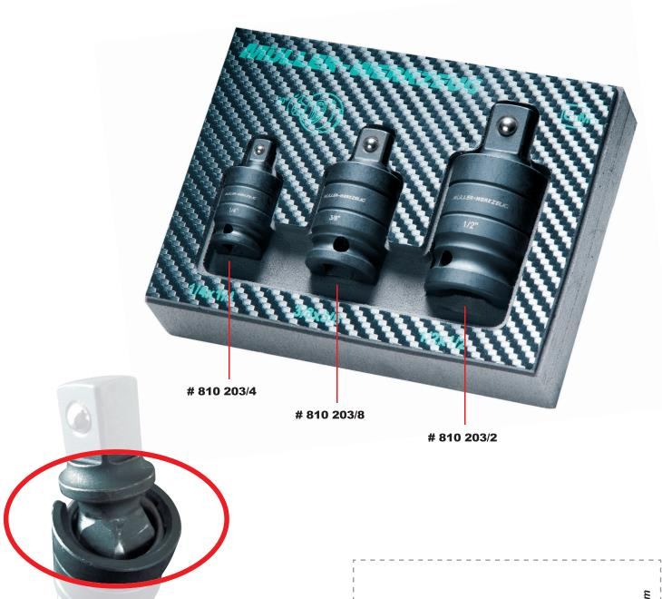
A no pin, impact adaptor set which includes 1/4", 3/8" and 1/2" adaptors. This set has a ball with flats, instead or a pin in oder to maximize torque transfer. It also reduces the chances of breaking. The pieces work as both a joint and straight connector.
