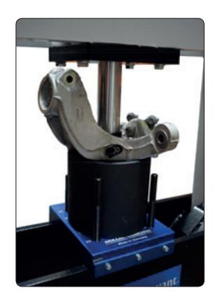
To be used in conjunction with the Universal Press Plate #432 650. This tool will help you press out wheel bearings by holding the hubs.
