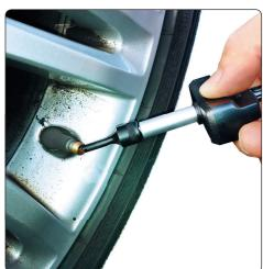
**Needed for mounting and demounting of the valve-type TPMS sensors.** These tools ensure that the sensitive TPMS-sensors parts such as the hex-nut or valve core will be tightened with the proper torque, which is required by the TPMS sensor manufacturer.
